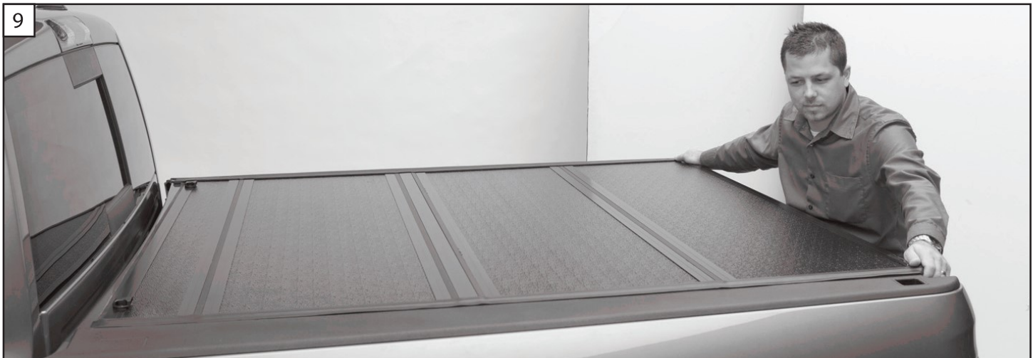
9. Test the rear latching assembly for smooth operation as this is the best indicator of the cover being positioned correctly. Be sure the latches on both sides are engaging with the cover mounting rail.
