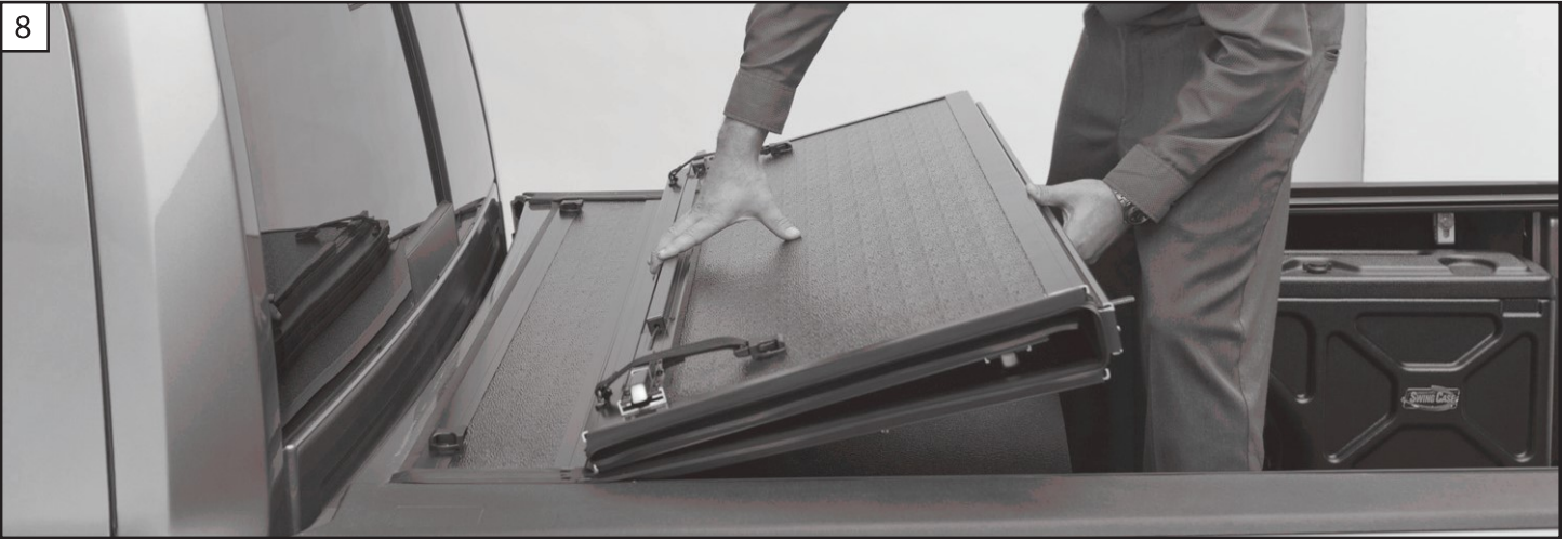
8. Carefully unfold the cover. Position the cover so it is centered side to side and front to back on the truck bed.
